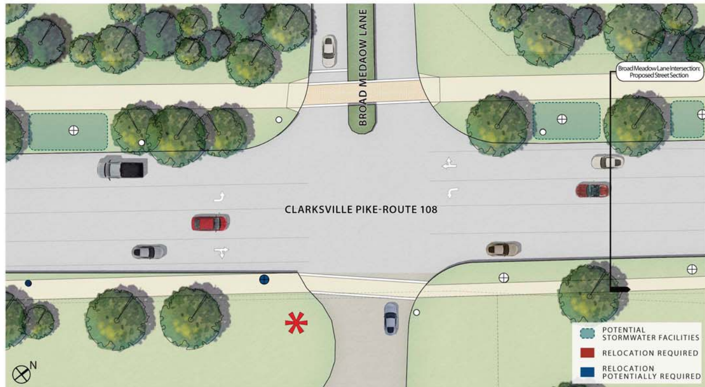
Proposed Streetscape: Streetscape improvements include crosswalks and ADA ramps, a continuous shared-use path (along the western edge of Clarksville Pike and in front of the schools on the eastern edge) and continuous sidewalks. Street trees are organically placed and clustered in keeping with the surrounding residential, school, and cemetery landscapes. Existing utility, signage, and traffic signal poles may need to be relocated.
