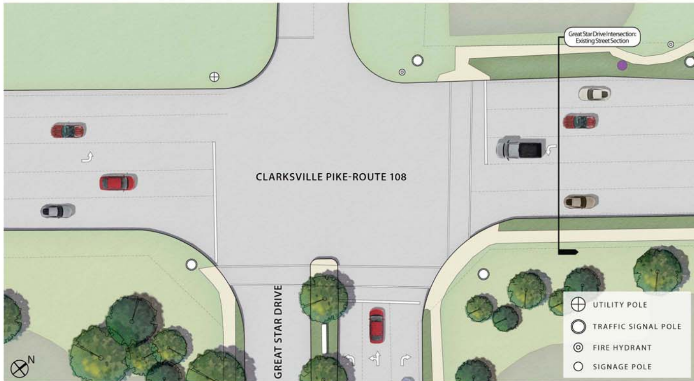
Existing Streetscape: The existing streetscape consists of intermittent sidewalks that jog to avoid existing utility lines. Striped crosswalks and ADA ramps exist in two locations only. Landscaping is minimal.
